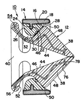
Figure 2A shows a heart valve assembly 10 with an occluder 12 disposed for movement within a valve seat assembly 14. Valve seat assembly 14 includes a soft seating ring 16, a rigid cast supporting ring 18, and a fixation cover 20. *Id.* at 3:51-64. Fixation cover 20 may be made of a Dacron mesh cloth and is initially secured to the heart tissue by suturing. *Id.* Thrombosis is then relied upon to retain valve seat assembly 14 in its proper position within the heart. *Id.*
