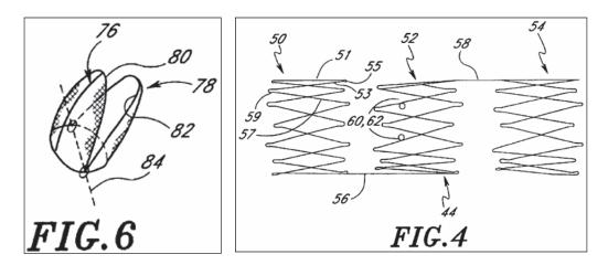
Shaolian further teaches that the center section 52 of the tubular wireframe 44, which is connected to the valve leaflets 76 and 78, can be connected to additional sections 50 and 54 by connectors 56 and 58 respectively. *Shaolian*, 6:60-62.
