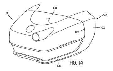
Connecting structure 100 includes conventional components such as housing 102 with a base portion 106 to support humidifier 30, a heater 152 to heat humidifier 30, a retaining portion 108 to secure connecting structure 100 to humidifier 30, and a retaining mechanism 140 to secure a CPAP apparatus to connecting structure 100. *See e.g., id.* at 9:30-35, 10:4-9, 34; 11:23-25.
