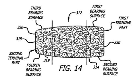
Figure 14, above, is a left side elevational view of a lordotic interbody spinal fusion implant. *Id.* at 5:11–12. The implant shown in Figure 14 has insertion end 320 and trailing end 330. *Id.* at 9:18–19. In addition,
