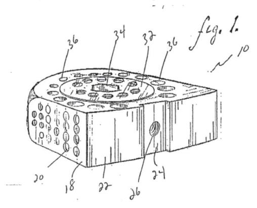
Figure 1, above, is a top right perspective view of the implant of Michelson '037. *Id.* at 10:13–14. The implant shown in Figure 1 has a substantially rectangular hollow configuration, and has a tapered forward portion. *Id.* at 11:30–32. Front wall 22 of the implant, is slightly convex,
