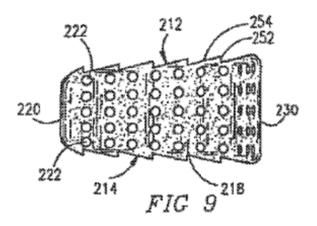
Figure 9 is a side elevational view of a lordotic interbody spinal fusion implant. *Id.* at 4:63:67. As seen in Figure 9, the ratchetings are oriented in the direction of the insertion end, 220, allowing for one-way insertion of the implant, and the bone engaging end, 252, prevents the implant from backing out once implanted. *Id.* at 8:40-49.
